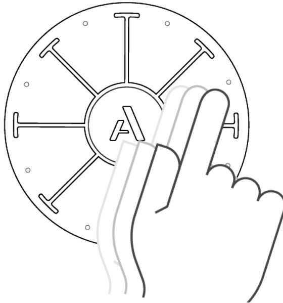
Press and move your finger within a pad, in and out from the center to the edge of Orba. Radiate effects Brightness. When using it with Orba's internal synthesizer it may be affecting volume, envelopes, and others effects. Try it in Bass and Chord modes to start.
