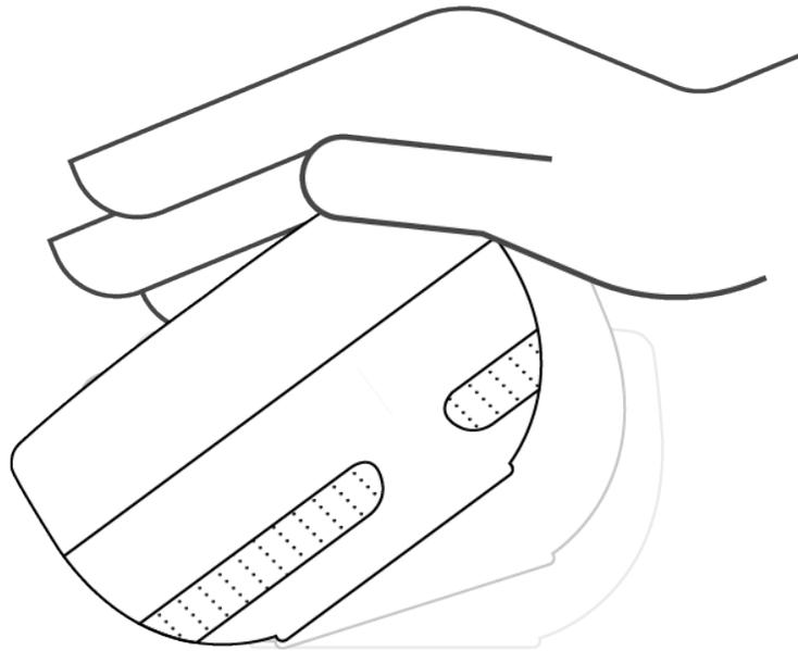
Tilt Orba to the side to play effects. Tilt is Orba's version of the mod wheel on a traditional keyboard controller. As mod wheel is a very common MIDI effect, you'll find Tilt works automatically with most software synths and apps.
