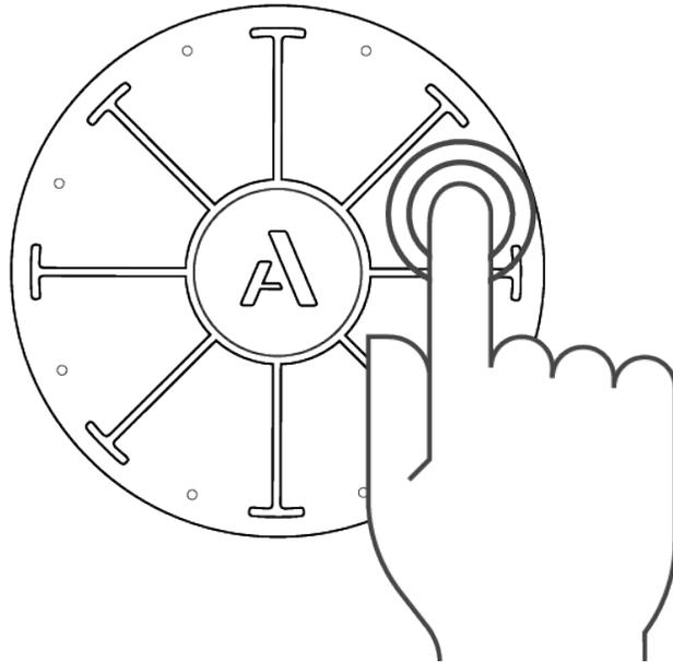
Tap and hold your finger on a pad with varying degrees of intensity. As opposed to velocity which detects pressure, Press is activated by making your finger take up more (and less) surface area. Think about it like this: the more you spread out your finger, the more Press is activated. Pressing with sustained pressure will modulate effects on Orba's synth.
