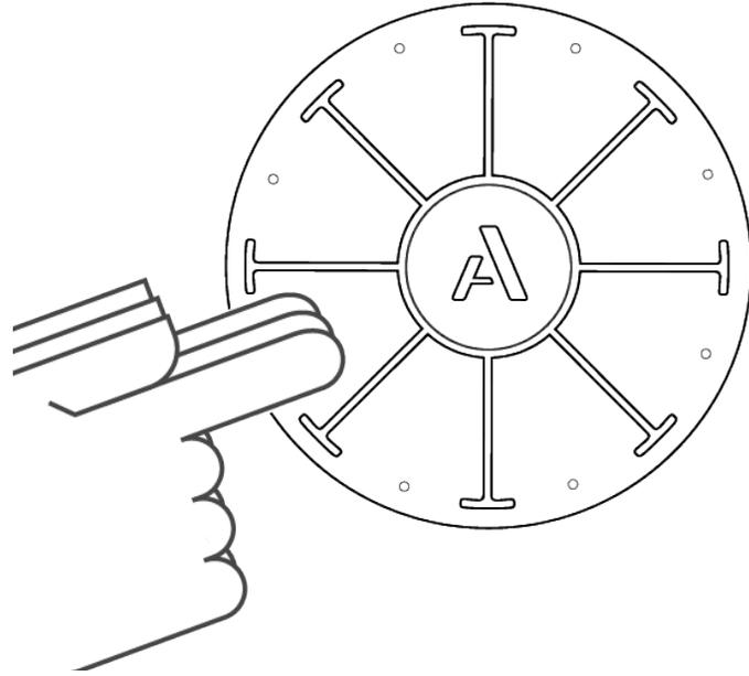
Tap and move your finger from side-to-side on a pad. Vibrato produces a change in pitch. the range of pitch can be adjusted with the Pitch Bend Scaling setting in the Orba App.
